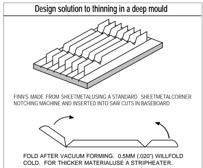
But if the rack dividers were vacuum formed flat and folded up afterwards, either cold or on a strip heater, they could be an insert in a casing made from another material.
