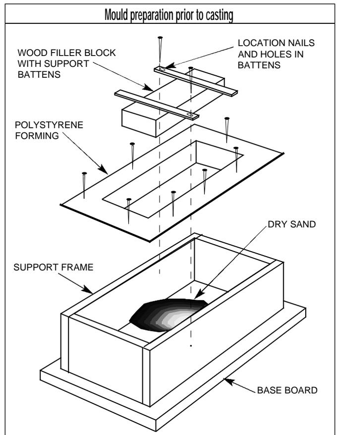
Turn the assembly back over, and you will have a sturdy hollow mould, that will not distort even under several kilos of resin or with the heat created by curing.
