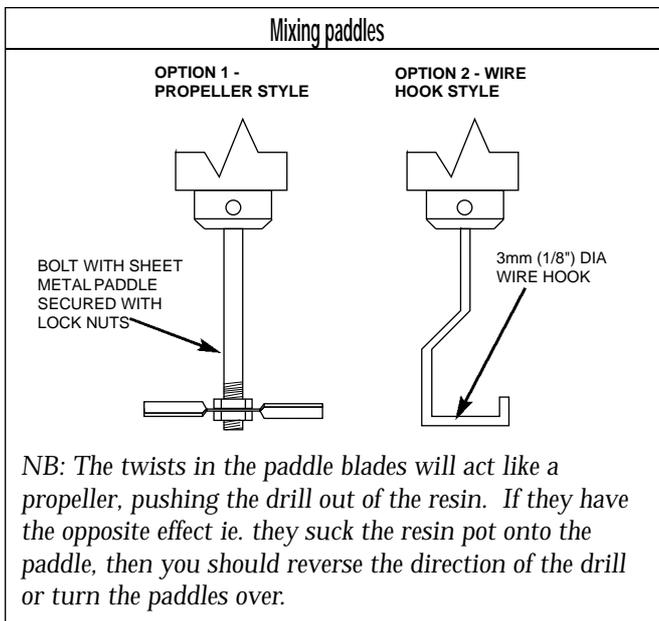
Most resins are too viscous to be mixed by hand so you will need to make some form of paddle mixer, fit it to an electric drill and mix for 3 - 4 minutes, making sure all the resin from the corners of the container is mixed in, to ensure you have a good resin that doesn't have any soft spots when it's cured.
