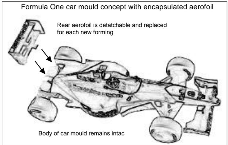
**VACUUM FORMING EXPANDED POLYSTYRENE**
