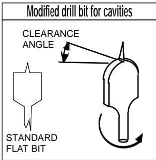
Dimples and hollows can be drilled into the mould using a custom shaped flat drill bit.
